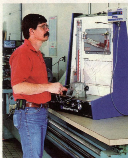
Things like velocity probes and other devices can be used with the bench. This means that not only can you measure the airflow inside the ports, but you can also start to understand it. When you start to understand and visualize airflow making power will become much easier to you. Picture courtesy of Superflow™.
